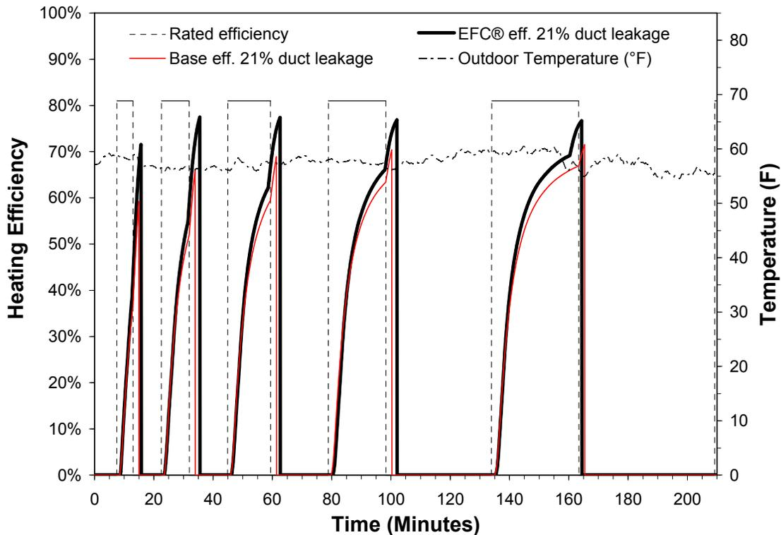
Figure 7 compares heating energy savings based on laboratory and field tests indicating similar results. Gas furnace heating energy savings based on field measurements with 21% duct leakage are calculated using regression Equation 6 based on the PLR.
